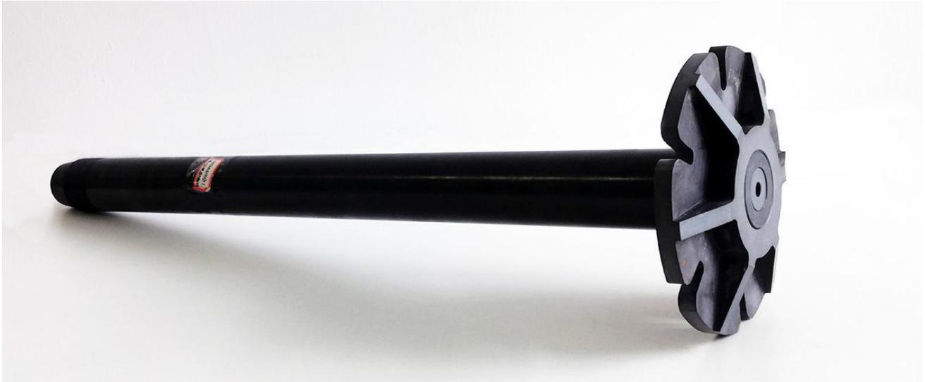
In order to remove hydrogen in the aluminum liquid, the silicon nitride hollow degassing rotor is used to feed nitrogen or argon, and the gas is dispersed by high-speed agitation, finally achieve the effect of neutralizing and discharging hydrogen.
