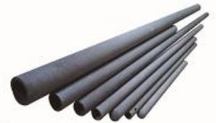
RSiC tubes including "Roller" "Furnace tube" & "Thermocouple Protection tube", With higher bending strength and no deformation under long term working temp 1650°C, RSiC life is much more than AL<sub>2</sub>O<sub>3</sub> tubes.
