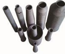
Re-SiC burner nozzle has excellent oxidation resistance & longer using life under 1650°C, no impurities appear (No-pollution on firing products) under super high temperature, it's an ideal kiln furniture as flame tubes in high temp fields.
