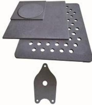
R-SiC loading plate has higher bearing capacity with small thickness. Higher bending strength & thermal conductivity, also no deformation & good oxidation resistance under 1650-1700°C, mainly as kiln furniture for kiln furnace in the industry of:
