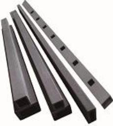
RSiC beam as kiln furniture widely used for loading structure systems of tunnel kilns, shuttle kilns and other industrial kilns. Higher strength & no deformation even in 1650-1700°C working temperature, also display longer life and excellent thermal conductivity make it save energy with less weight of the kiln car. applied following industries:
