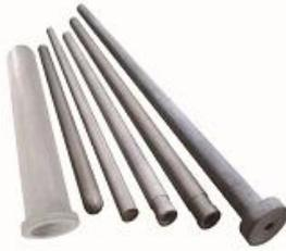
NSiC material has very excellent resistance of molten metal corrosion, as thermal couple protection tube in temperature measuring system, or electrical heating protection tubes in metallurgy process, which can directly touch with the liquid-metal, high strength & longer life.
